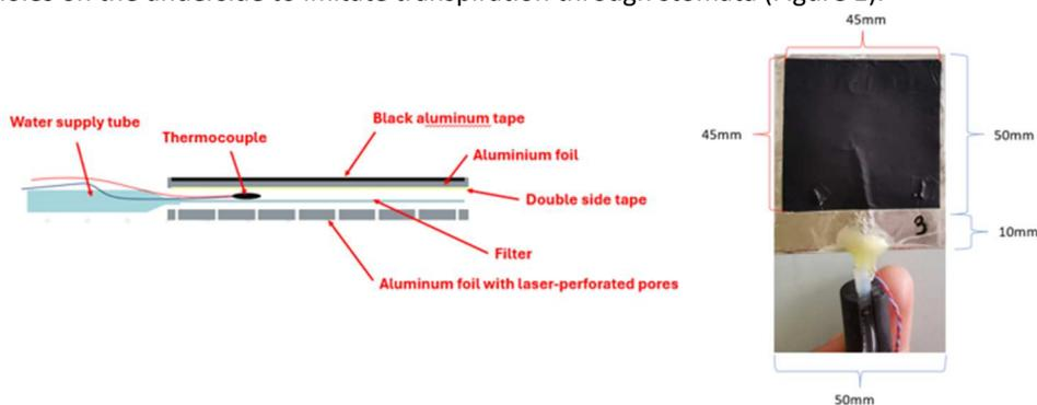
Figure 1. Leaf replica design scheme and a photo with the dimensions
